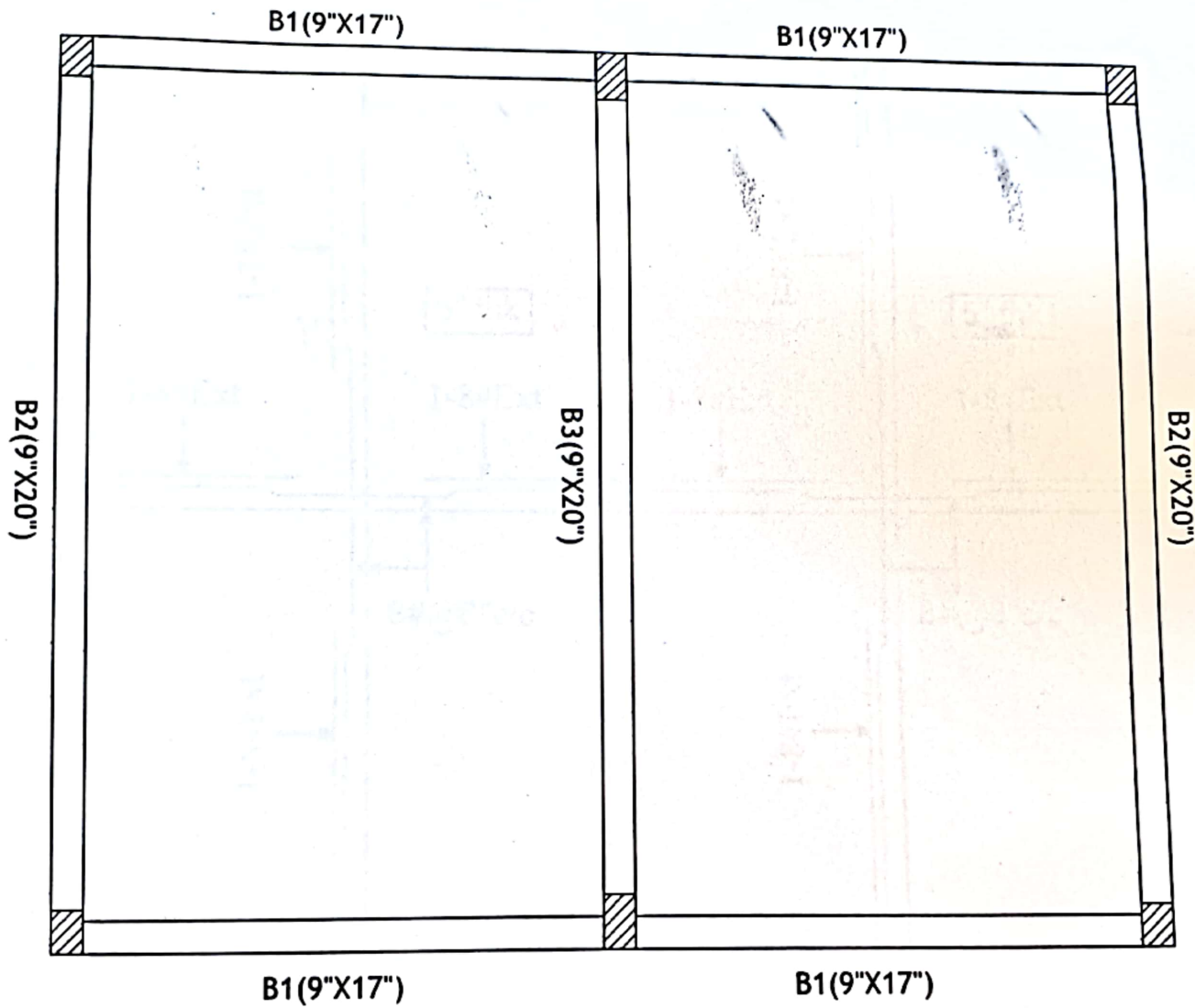
ROOF BEAMS FRAMING LAY OUT
